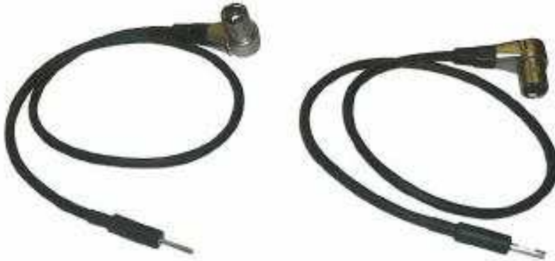
Figure 4: Left Hand and Right Hand Connection Leads. Used to Connect the DCVG Meter to the Probe Handles
