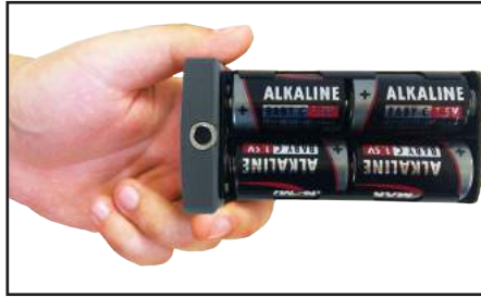
Install the batteries, observing the polarity
