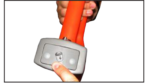
Install four new elements into the battery compartment of the device, minding polarity. Install the battery compartment into the body until it snaps.
