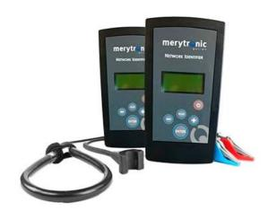
The device consists of a transmitter (IC2G-TX) and a receiver (IC2G-RX), and it is easy to use: the transmitter (TX) is connected to an LVdistribution cable and the receiver (RX) is used to identify or locate that cable upstream, towards the MV/LV transformer.
